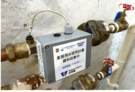
(a) Sensor node with waterproof box
