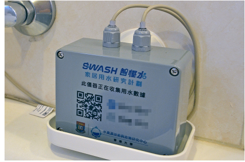
(b) Waterproof box containing the printed circuit board and battery pack
